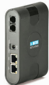
SETU ATA2S 2-FXS Ports, 1-WAN Port, 1-LAN Port and 3-SIP Accounts
